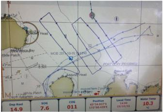
Electronic aids such as GPS provide navigational data in relation to the seabed not the surface of the sea. The course taken by the CRV through the water will be influenced by wind and current and search patterns will appear distorted.
